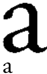
8-3 Enlargement of a screen display of an a shows the “jaggies” caused by pixels.
